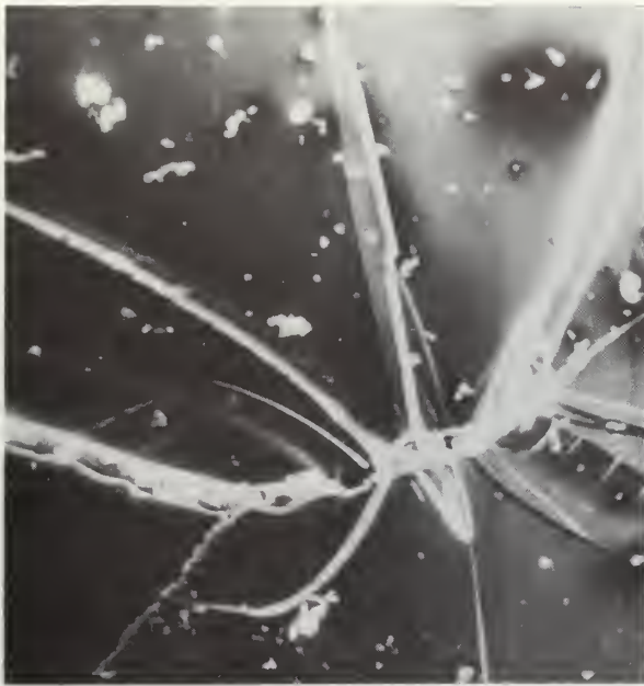
FIGURE 16. SCANNING ELECTRON MICROGRAPH OF THE FRACTURE SURFACE AT A FLAW OF A TENSILE SPECIMEN; EPON 828 + 10 pph CTBN 20-64 (SMALL PARTICLES) + 5 pph CURING AGENT D.
